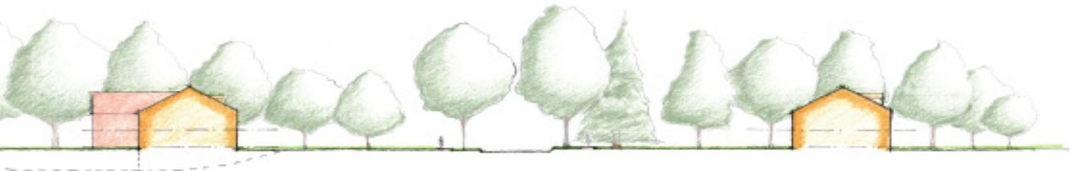
Figure 1. Typical street section. Note the deep setbacks, mature street trees, and abundance of yard trees (front, back, and side). The dashed line on the house to the left shows a condition in which the grade slopes down to a basement-level garage.
