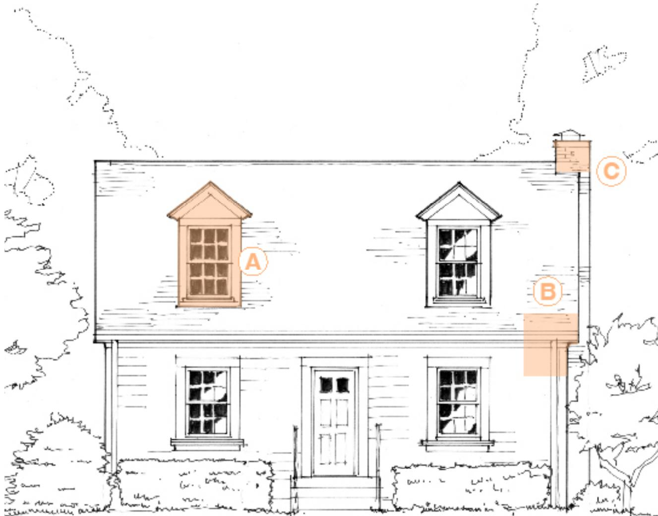
A. DORMER: Double-hung windows with 6-over-6 lite/muntin pattern. The windows maintain the same proportion, 2:3, as the windows below. The dormer roof pitch has a slope less than 12:12. For more dormer details, see pages 110-115.
