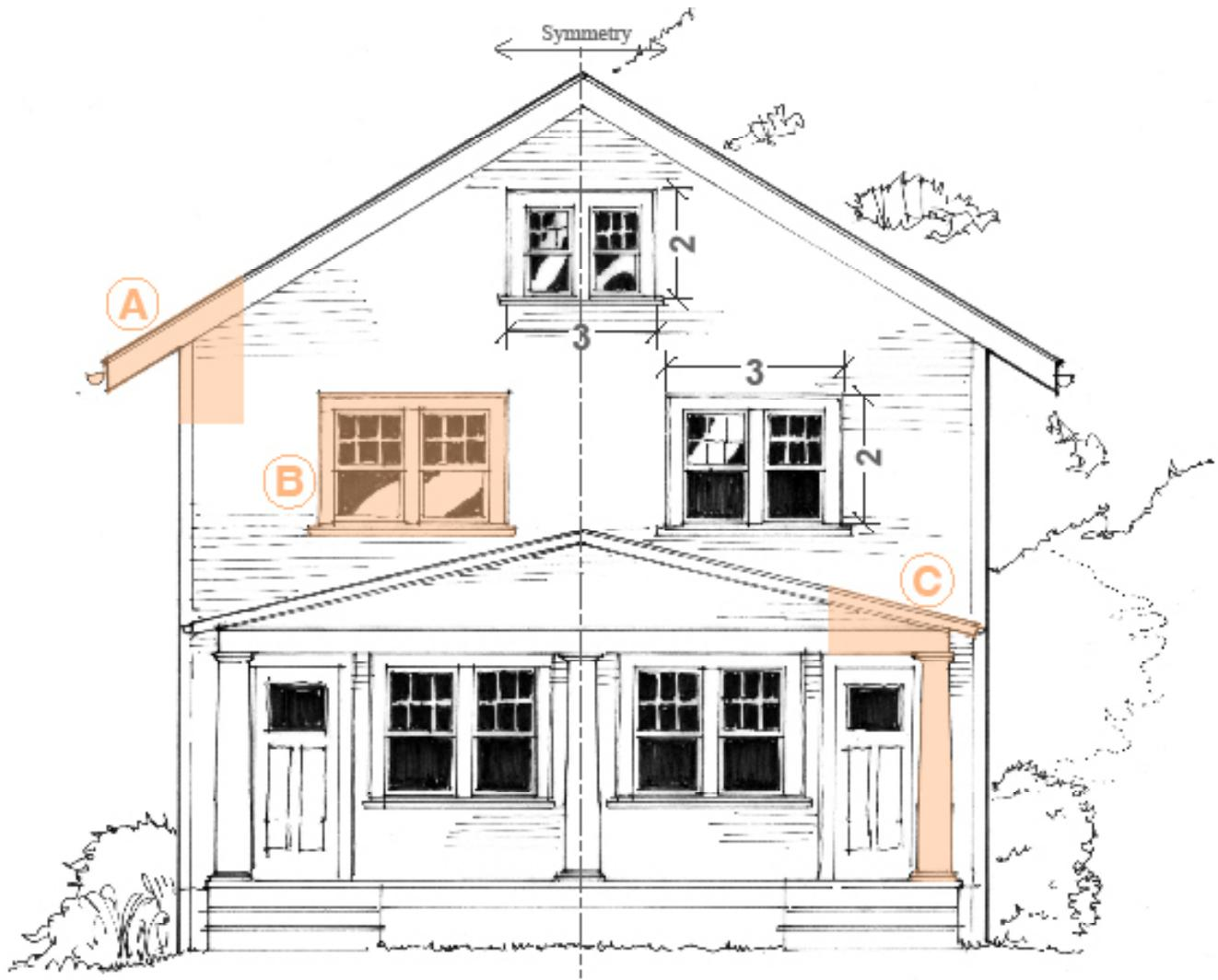
A. EAVE: Note eave is deeper in this example. Boxed-out eaves are not used. For more eave details, see pages 90-95.
