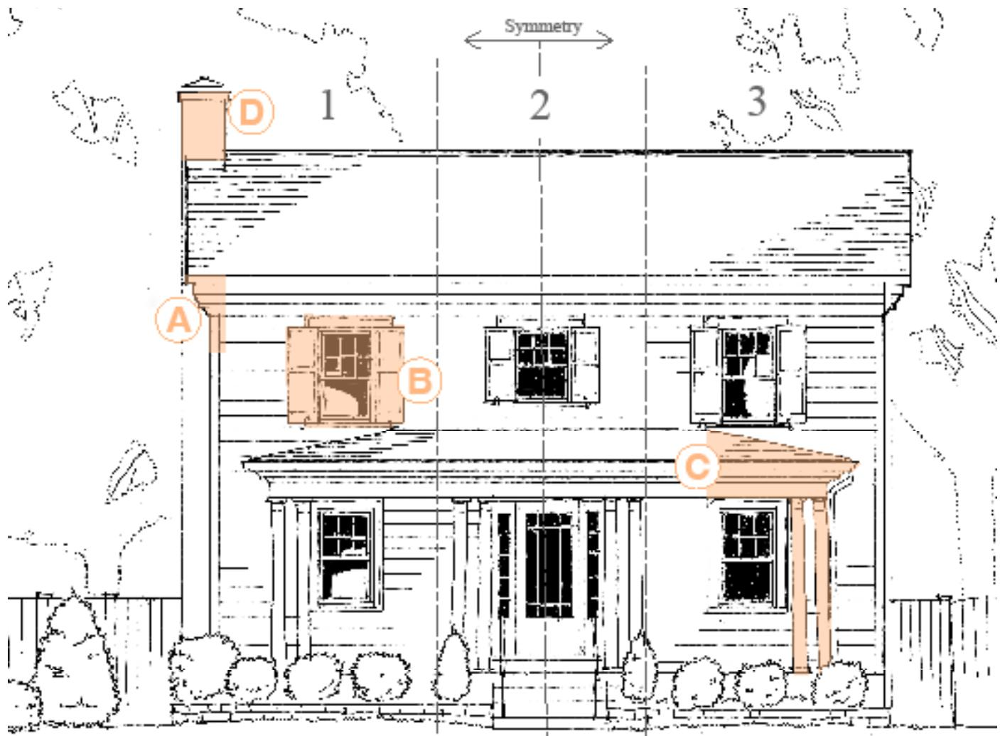
**A. EAVE:** The length of the main roof eave overhang is equivalent to the height of the fascia and the frieze board. For more information on eaves, see pages 90-95.
