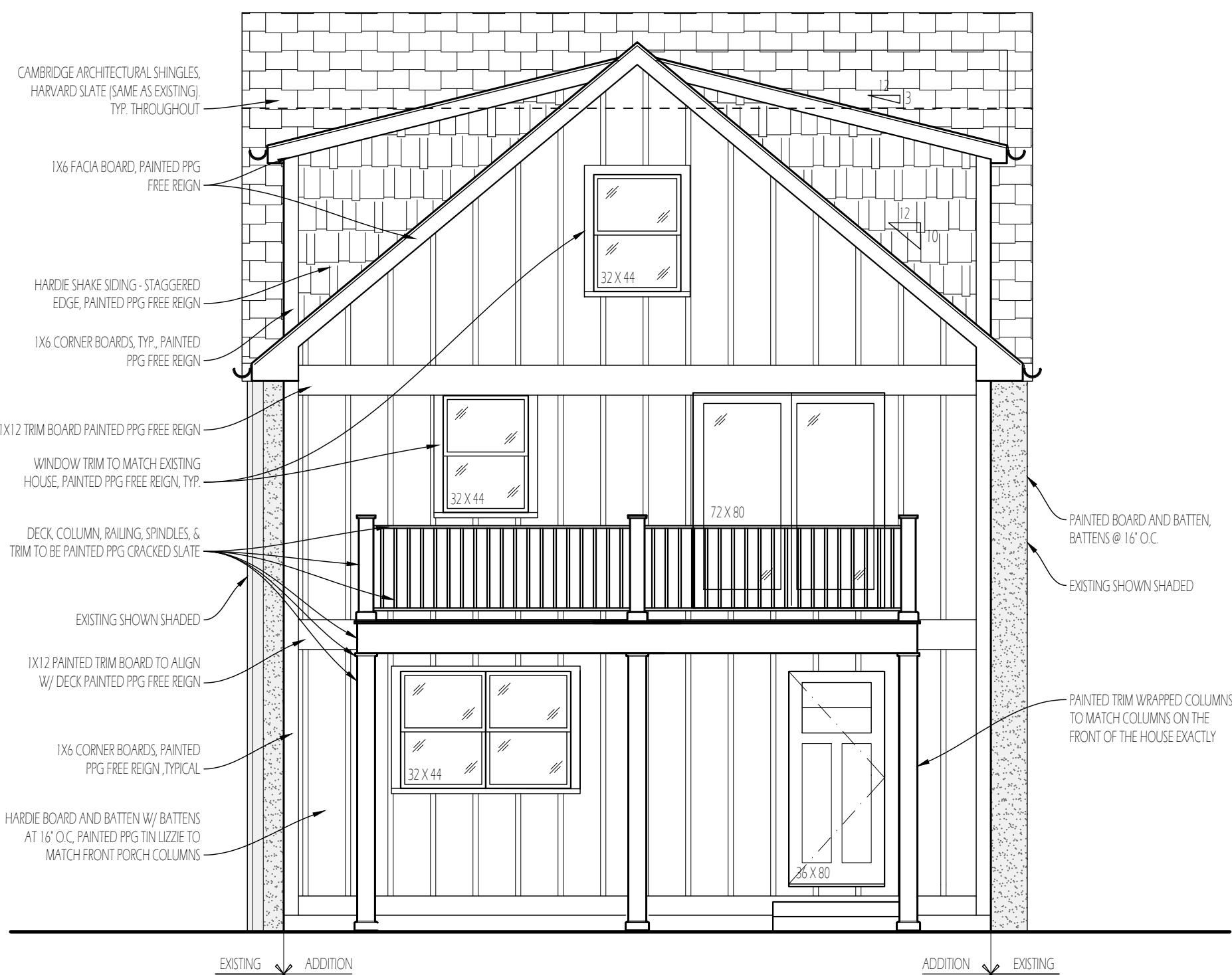
REAR EXTERIOR ELEVATION OF ADDITION SCALE: 1/4" = 1'-0"
